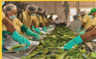
After removal from the plants, the leaves are transported to an on-site processing station where they are washed twice before being filleted by hand. This ensures the rind is fully removed and only the nutritious inner leaf gel is left.
